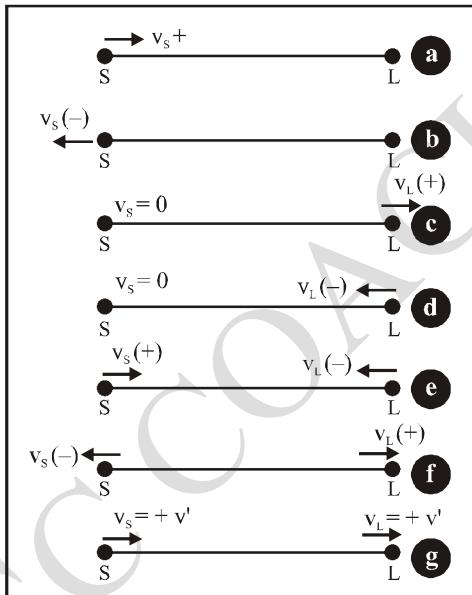
$$v' = \frac{(v - v_L)}{v} v \quad \text{i.e. } v' < v$$
